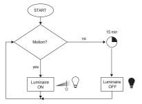
Note: If the luminaire is switched off manually using the pushbutton, the luminaire will not switch on again automatically via the motion sensor until after a period of 1 minute elapses. After this period expires, the next motion switches the luminaire on.
