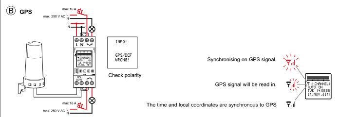
During normal operation the GPS-signal is actively decoded every 6 hours for 30 minutes. The time zone is not synchronised. A manual adjustment is necessary. By activating the expert mode the resolution of the coordinates can be increaded from degree to minute
