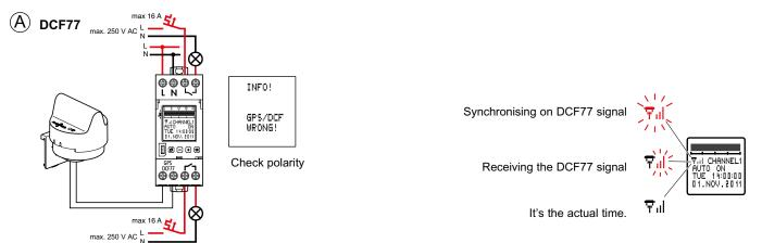
During normal operation, the DCF77 signal is actively decoded every 6 hour for 30 minutes.
