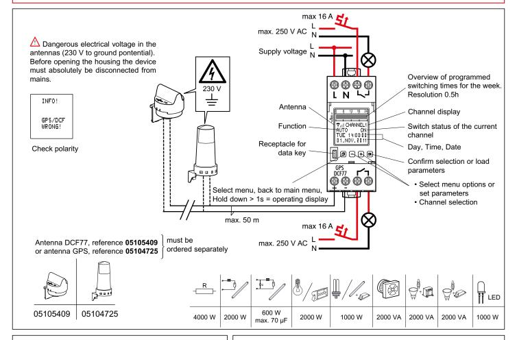
Operating principle: Type 1.B. S/R. T. IEC/EN 60730-1, IEC/EN 60730-2-7 Operation in a normal environment
