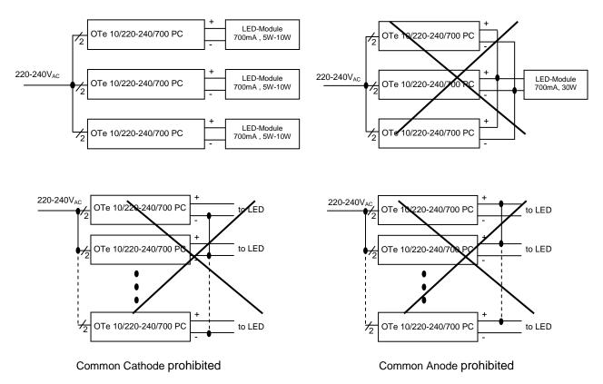
The installation of two or more OPTOTRONIC<sup>®</sup> OTe 10/220-240/700 PC Power Supplies with common "-" or "+" wiring by the intention to save wire to LED modules is prohibited, in order to avoid exceeding the maximum allowed system touch current levels on the accessible parts of the installation.
