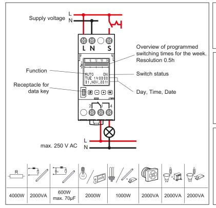
Operating principle: Type 1.B. S. T. IEC/EN 60730-1, IEC/EN 60730-2-7 Montage: in distribution panel, Degree of contamination: 2 Switch output, potential-free Rated impulse voltage: 4 kV
