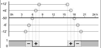
If the offset setting is in degrees the time switch switches on and off at times of equal brightness, despite the differences in twilight time lengths over the course of the year.
