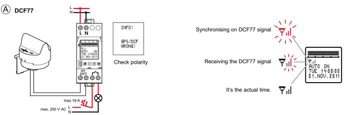
During normal operation, the DCF77 signal is actively decoded every 6 hour for 30 minutes.
