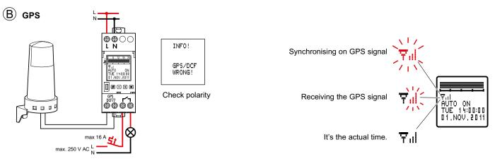
During normal operation the GPS-signal is actively decoded every 6 hours for 30 minutes. The time zone is not synchronised. A manual adjustment is necessary. By activating the expert mode the resolution of the coordinates can be increaded from degree to minute
